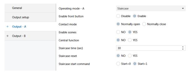
As shown in the figure above, the parameters on the switching output setup page are as follows:
